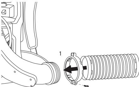
2. Orient the alignment markers to face each other (2). Insert and tighten the hose clamp screw.
