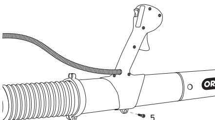
6. Secure the throttle cable onto the clips on the two hose clamps (6).
