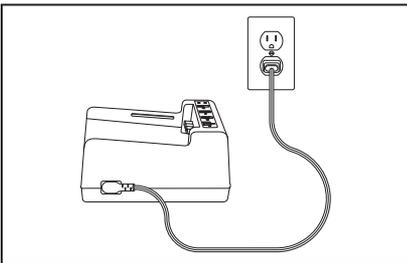
Only use the cord set that was supplied with the charger. At first use, verify that the plug type matches the receptacle.
